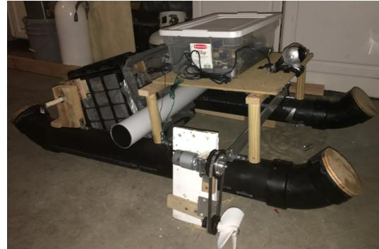
system, and added caulking to places that were vulnerable. This design was much easier to build and not very expensive. The final design sufficiently protects the sensitive electronics, is able to carry 36 kilograms of weight, and has ample space to expand. However, this frame is not as sturdy as it should be.
